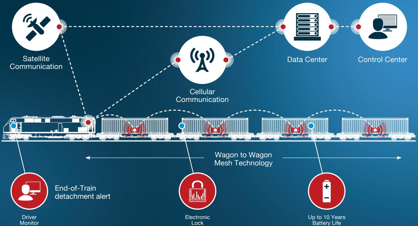
A unique small, ruggedized transmitting tag with patented mesh technology is affixed to each wagon. Due to unique technology the tags can transmit for up to 10 years. A smart Telemetry controller is installed on each locomotive and creates a communication chain between all wagons and the locomotive.
